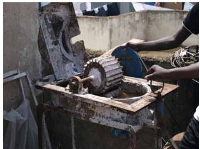
A pulping machine used to make sanitary pads from water hyacinth (Photo: Lars Marcus Vedeler)
